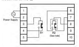
\* 2. Contact symbol is shown as because it is possible to change relay R2 between time-limit contact and instantaneous contact.
