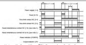
Note: t is the set time, Rt' is the reset application time, and t is the power interruption time.
